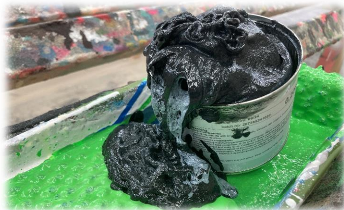
When too much resin hardens at once....
